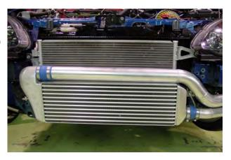
(5) Install the Intercooler pipe I-5 to the I-4 as shown. Secure the I-5 to the body. Modify the splash guard where it contacts these pipes.
