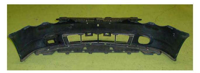
\* Cut the bumper little by little and test fit on the vehicle. Trim the area the hits the intercooler.
