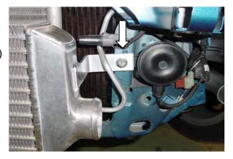
(4) Position the intercooler so that it is mounted straight before tightening the bolts.
