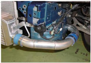
(4) Install the I-3 to the intercooler outlet as shown.
