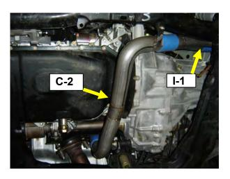
(2) Install the I-2 pipe between I-1 and intercooler inlet as shown.
