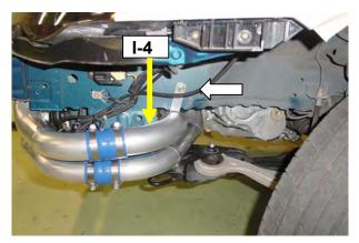
(6) Install the Compression pipe C-4 from the turbo kit between the pipe I-5 and the throttle body as shown. Reuse the hoses and clamps from the turbo kit.
