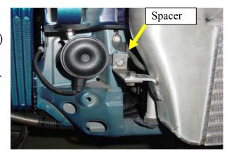
(3) Secure the right side of the intercooler to the body as shown using the provided spacer between the horn bracket and I/C bracket.
